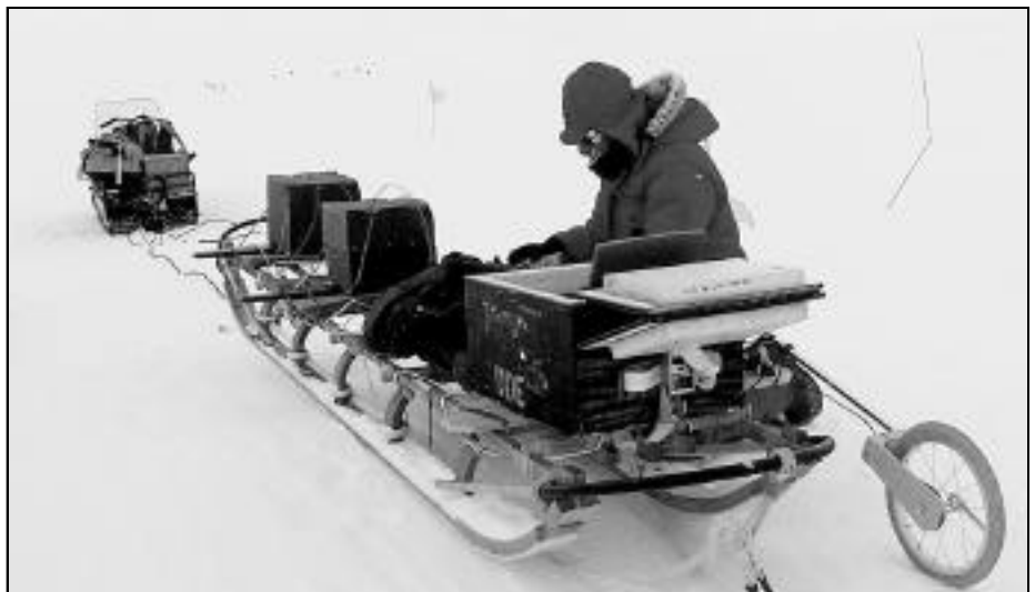
Charlie Raymond makes final adjustments to a Nansen sled that carries radar equipment. Raymond used this high-frequency, short-pulse radar to look at the near surface layers of snow near the summit of Siple Dome. The small attached tire sends ground distance measurements to the computer inside the open box.
