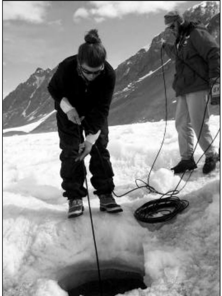
Researchers Laura Spinney, left, and Craig Wolf lower a profiling natural fluorometer 18 meters to the bottom of Lake Hoare to measure the amount of incoming natural light from the surface as well as fluorescence from algae.
