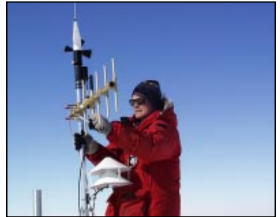
Steve Clark attaches a directional radio antenna to an automated weather system. The small, remote weather observatory transmits temperature, humidity and windspeed data every 15 minutes. Photo by Jeff Inglis.
