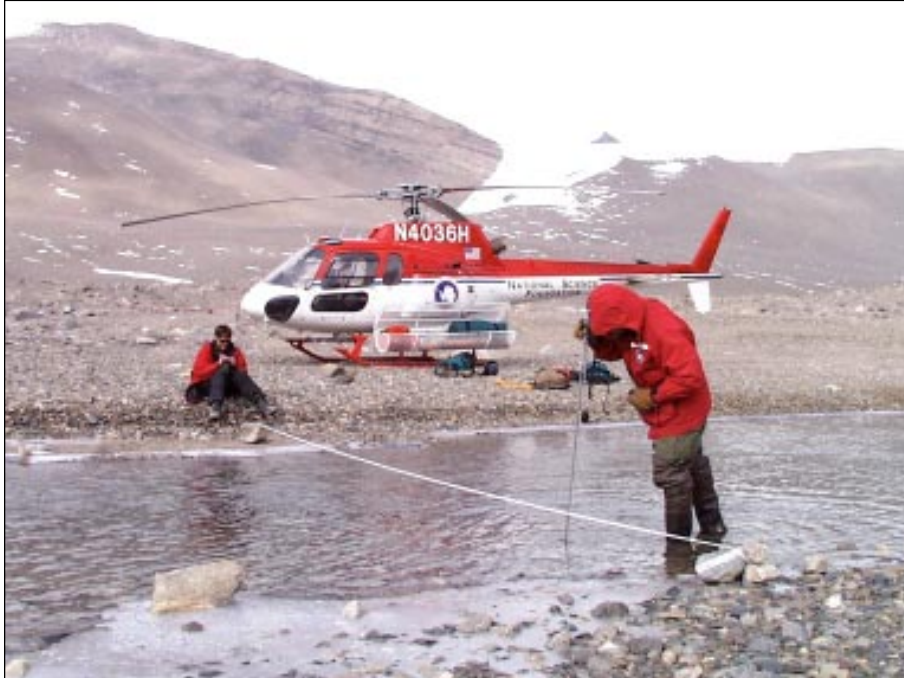
Ethan Chatfield records data as Mike Gooseff measures the depth and velocity of the Onyx River. The Stream Team is responsible for monitoring 18 sites in the Dry Valleys. Photo by Josh Landis.
