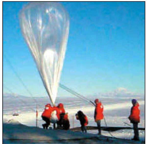
A team of scientists and engineers launch a balloon loaded with instruments that measure ozone. Photos courtesy of Terry Deshler.
