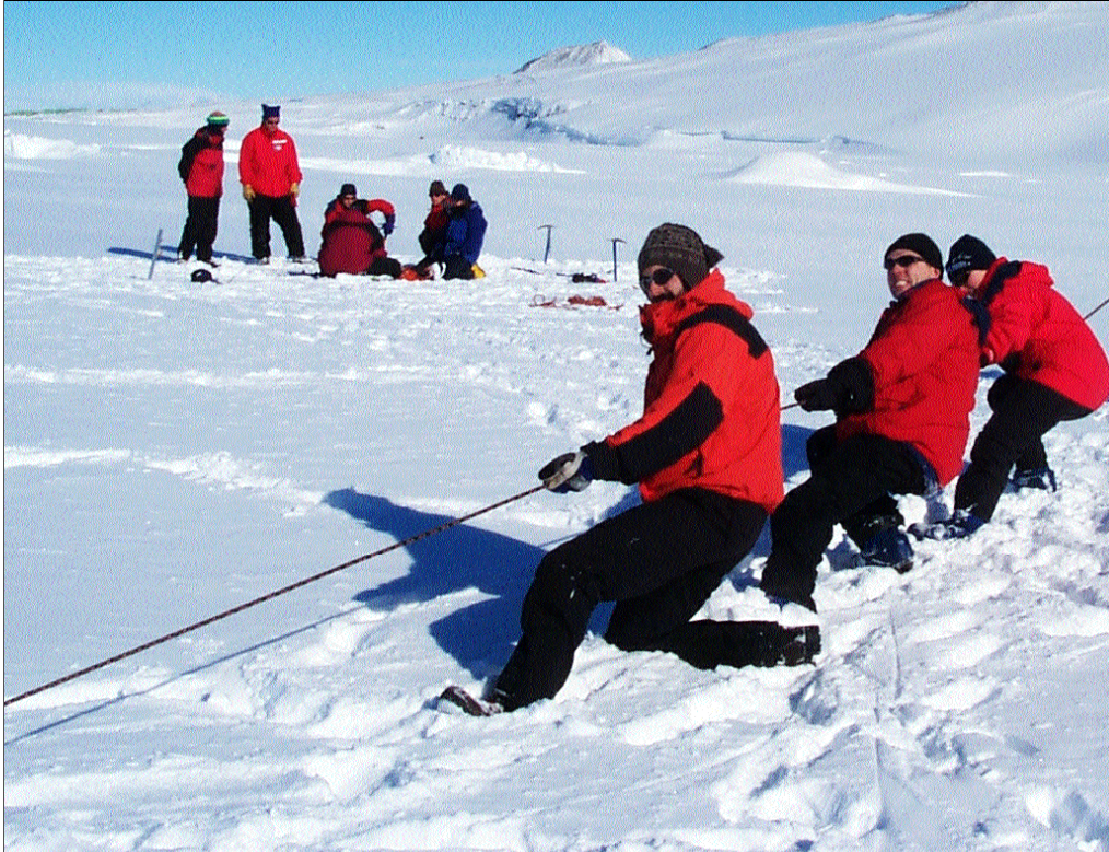
Justin Reese, Joe Harrigan and M.K. Fortune test a snow anchor during tryouts for the secondary search-and-rescue team. The so-called "dead man" device is buried in the snow to secure a crevasse rescue line. Twenty-eight people tried out for the team, which has 12 spots. Photo by Tobias Schunck.
