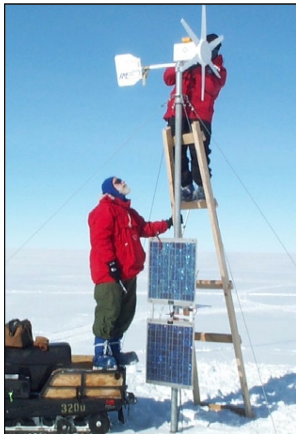
Don Voigt, bottom, and Sridhar Anandakrishnan work on the wind generator at the Siple Dome site. A combination of solar and wind energy powers the equipment and keeps it warm enough to function. Photo by Jerry Bowling.
