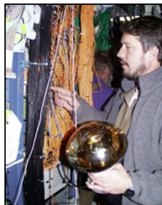
Steve Barwick holds a neutrino detector. About 640 of these are buried in the two-mile thick ice cap at the South Pole.
