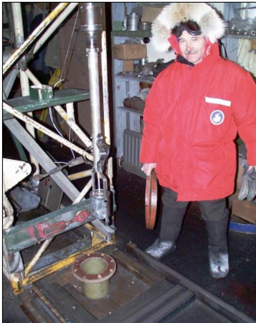
Russian driller Valery Shoshkin stands at the top of the two-and-a-quarter-mile deep hole over Lake Vostok. The bottom of the hole is about 300 feet from the lake's surface. Photo by Josh Landis.
