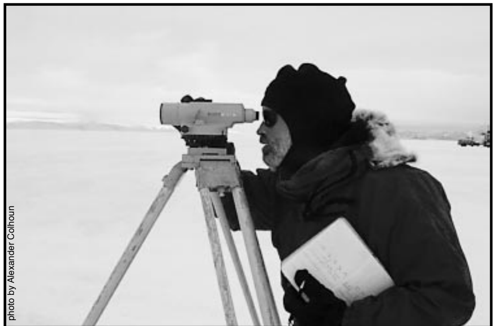
Jeff Scanniello, an OAE, adjusts an auto level as he surveys the ice runway before a C-141 lands.
