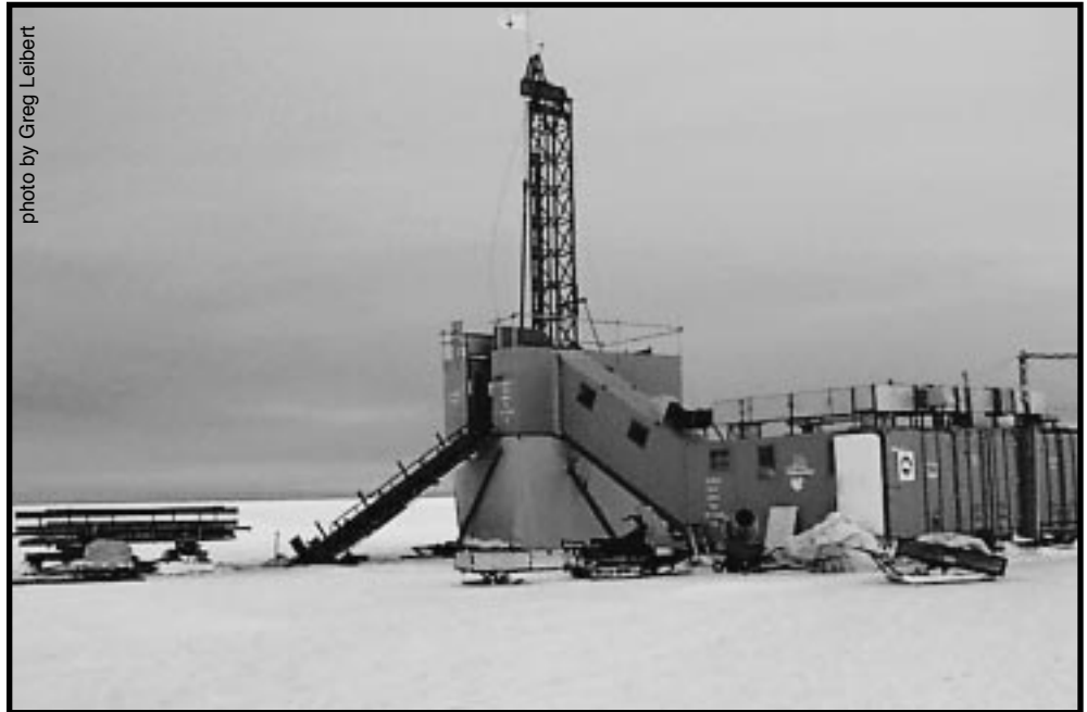
The Cape Roberts Project drilling rig sits on 1.5 meters of ice, just one-tenth of a meter more than the minimum required to support the five-ton platform.
