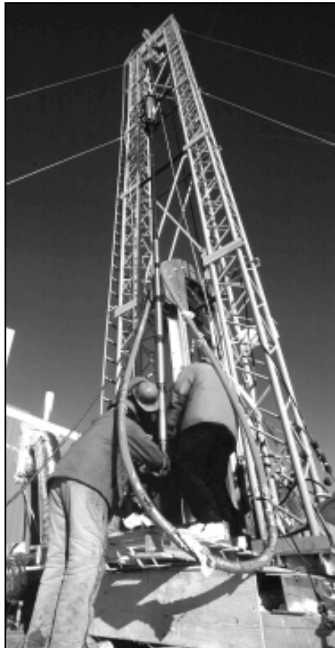
Drillers from the Polar Ice Coring Office use hot water hydraulics to bore holes more than a mile deep. Photo courtesy of Paul Bellrichard.
