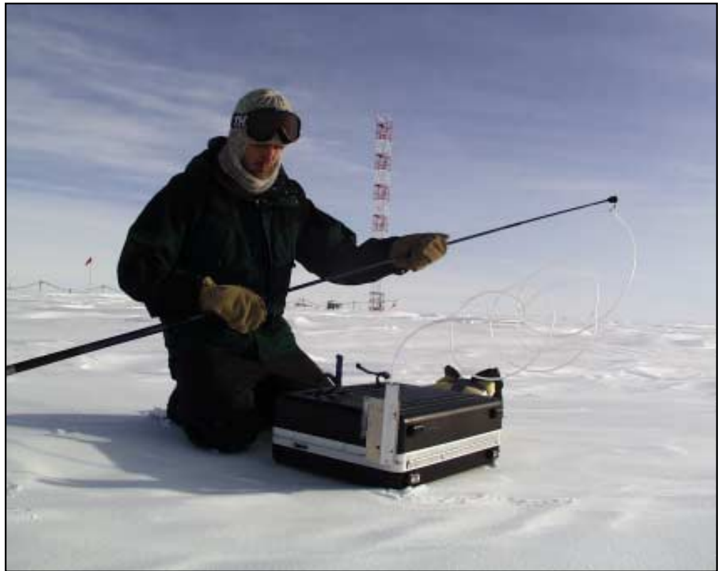
NOAA researcher Don Neff prepares to take a gas sample in the Pole's Clean Air Sector last month. The sample will be sent back to a laboratory in Colorado for analysis. Photo by Aaron Spitzer.
