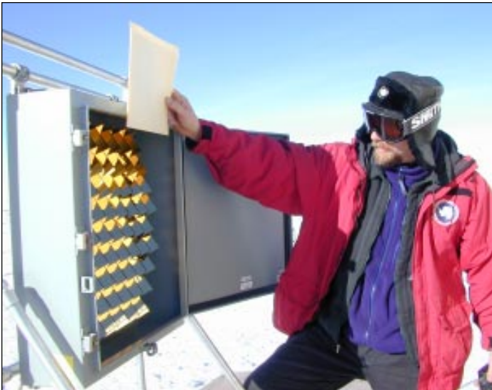
Von P. Walden checks the dimensions of an infrared beam on a reflectometer. The equipment helps measure the absorption of infrared radiation by water vapor in the atmosphere. Photo by Jeff Inglis.
