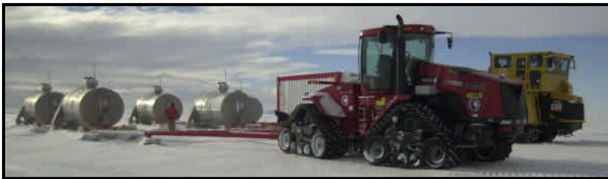
A Y-shaped tongue attaches fuel sleds to the tractor that will pull them on the traverse, allowing the sleds to glide on either side of the tractor tracks.
