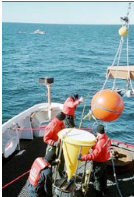
Walker O. Smith Jr. / Special to The Antarctic Sun A mooring is in the process of being deployed during an IVARS research expedition. The instrument in the foreground is a time-series sediment trap, which collects sinking particles over set time intervals. The ball is a float that keeps the mooring taut in the water column.
