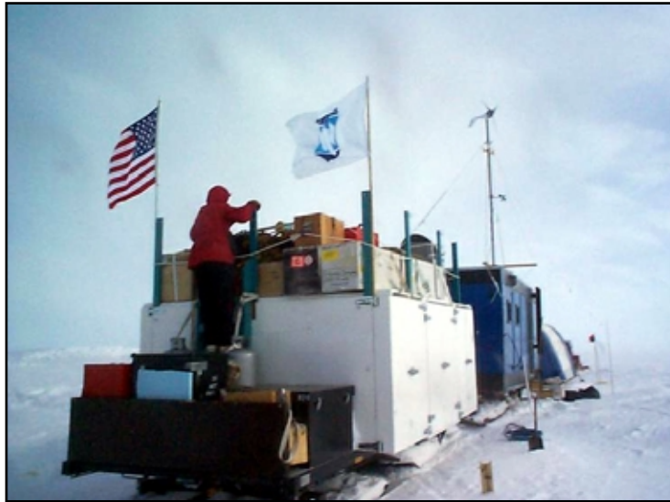
A member of ITASE loads boxes on top of the ice core freezer, the first component of the train. The next building in the convoy is the bunk house, followed by the kitchen. Photo by Bob Zook.
